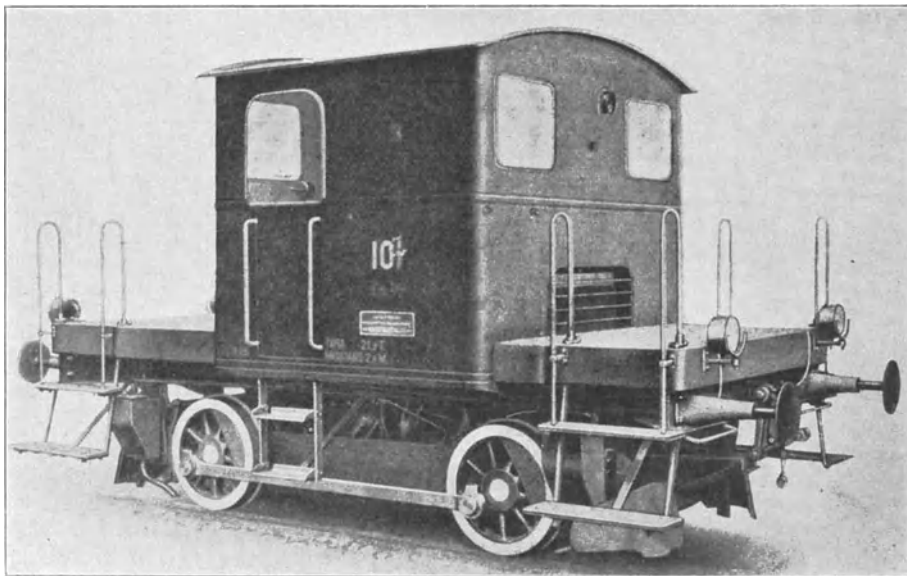
Fig. 55. Shunting locomotive Swiss Federal Railways.
