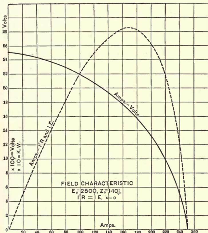
Fig. 129. Field Characteristic of Alternator on Non-inductive Load.
