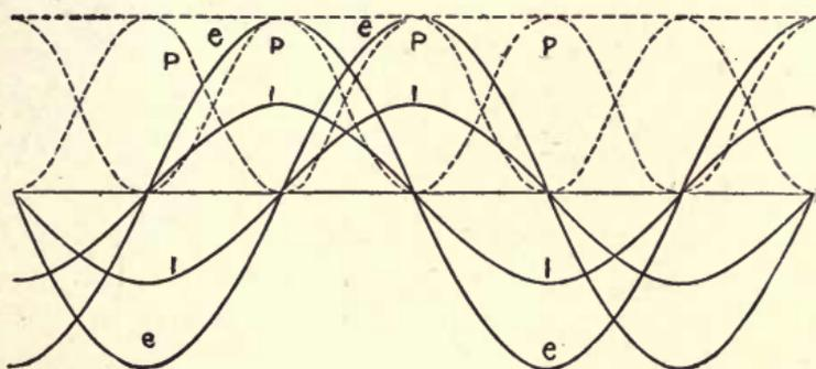
Fig. 187. Quarter-phase System on Non-inductive Load.
