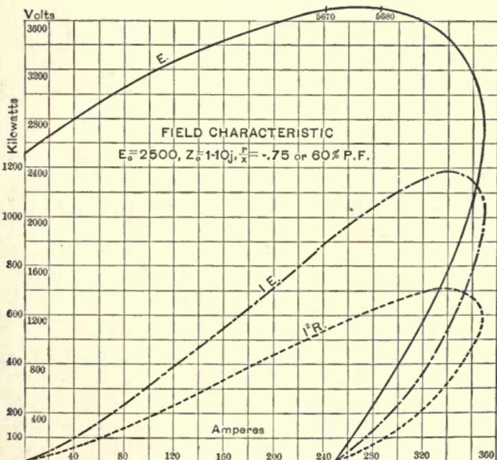
Fig. 132. Field Characteristic of Alternator, at 60% Power-factor on Condenser Load.
