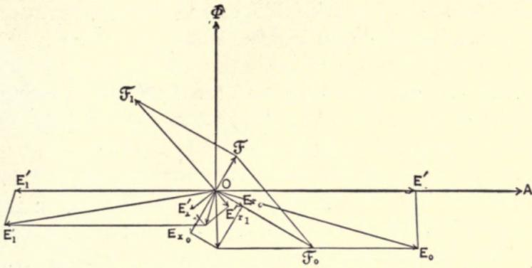
Fig. 100. Transformer Diagram with 50° Lead in Secondary Circuit.
