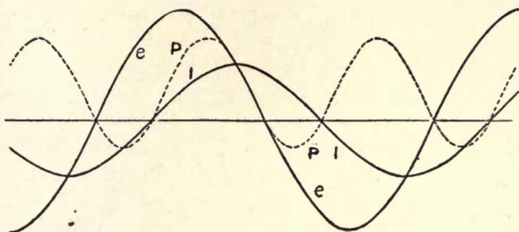
Fig. 186. Single-phase System on Inductive Load of  $60^\circ$  Lag.
