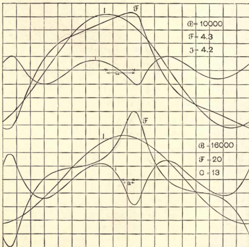
Figs. 68 and 69. Distortion of Current Wave by Hysteresis.
