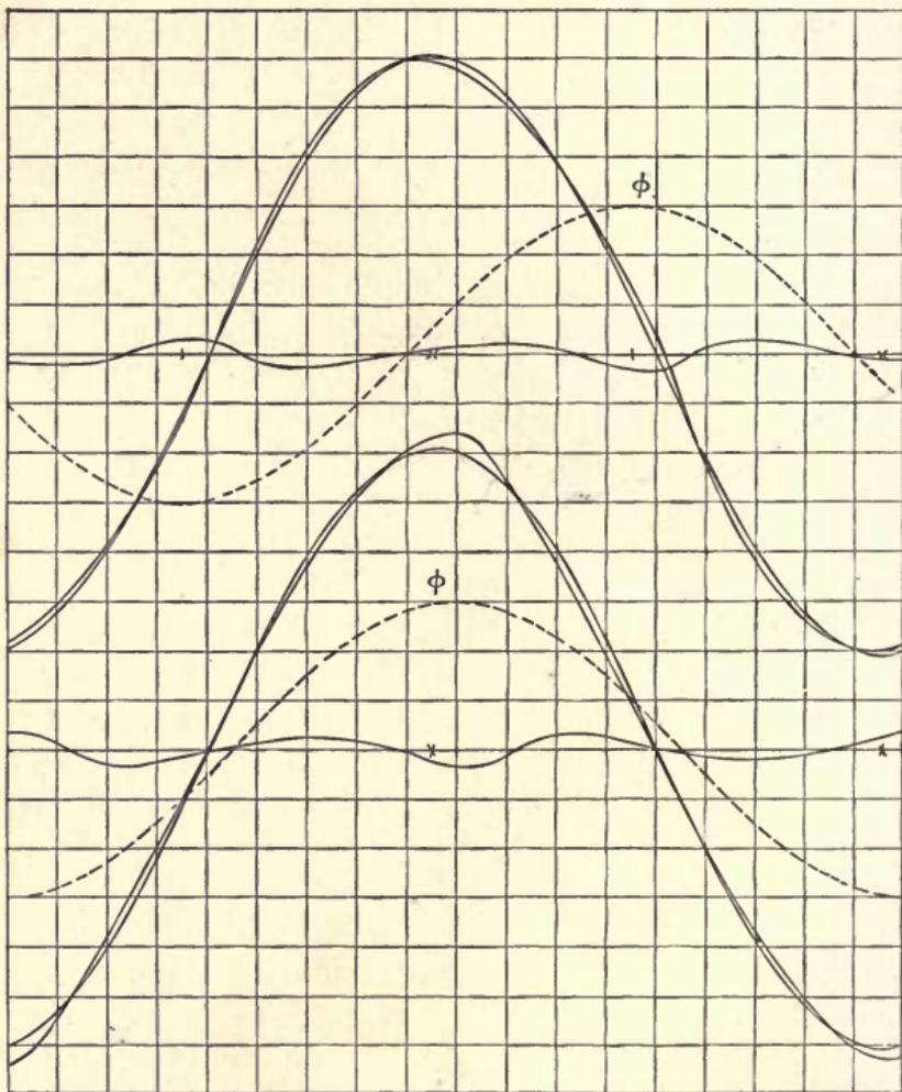
Figs. 70 and 71. Distortion of Current Wave by Hysteresis.
