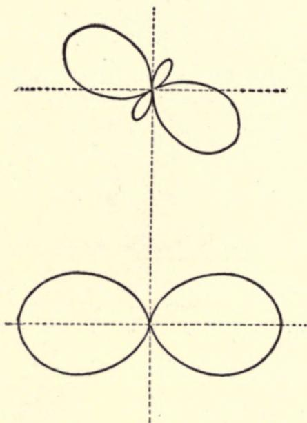
Figs. 193 and 194. Power Characteristic of Single-phase System, at  $60^\circ$  and  $0^\circ$  Lag.
