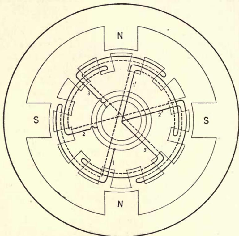
Fig. 178. Three-phase Star-connected Alternator.
