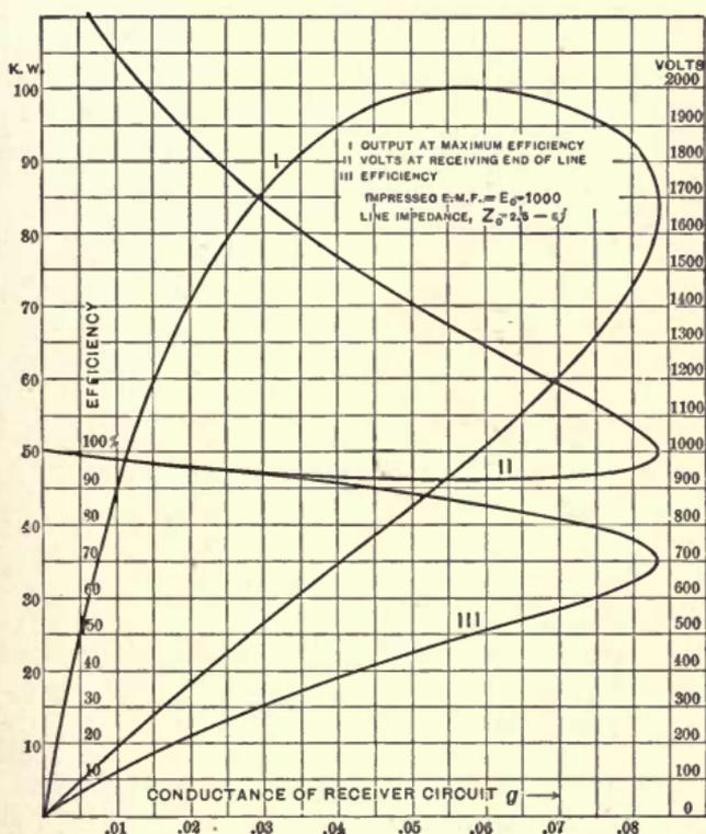
Fig. 60. Load Characteristic of Transmission Line.
