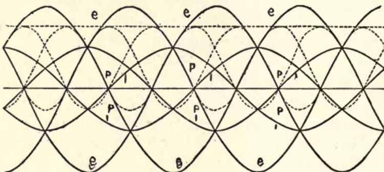
Fig. 190. Three-phase System on Inductive Load of  $60^\circ$  Lag.
