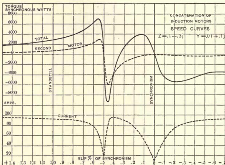
Fig. 124. Concatenation of Induction Motors. Speed Curves.
