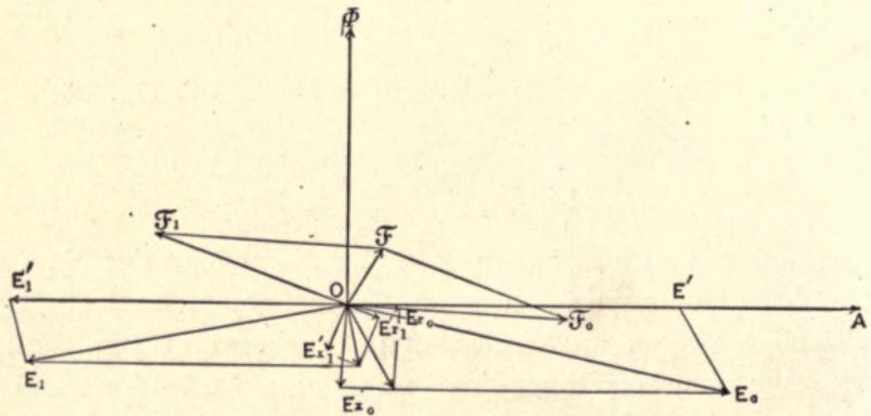
Fig. 99. Transformer Diagram with 20° Lead in Secondary Current.
