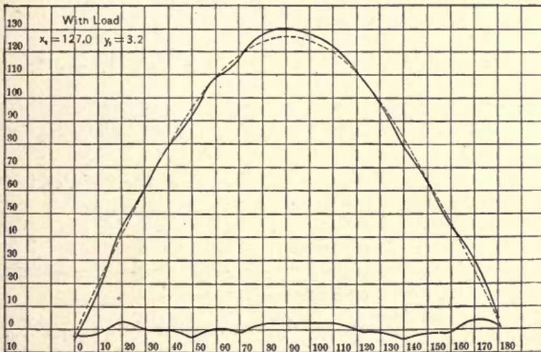
Fig. 170. Full-Load Wave of E.M.F. of Multitooth Three-phaser.
