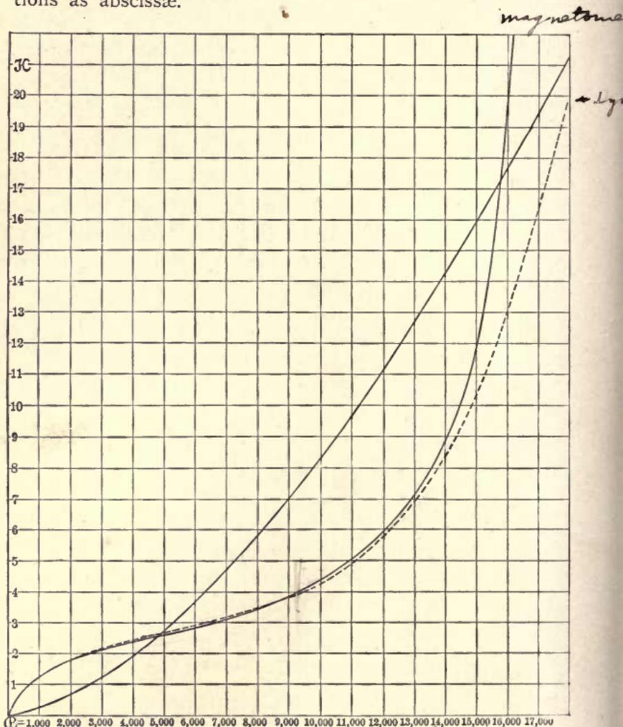
Fig. 72. Magnetization and Hysteresis Curve.
