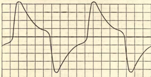
Fig. 2. Wave without Even Harmonics.
