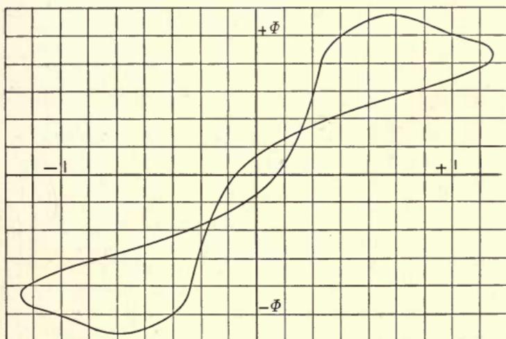
Fig. 166. Hysteretic Loop of Reaction Machine.
