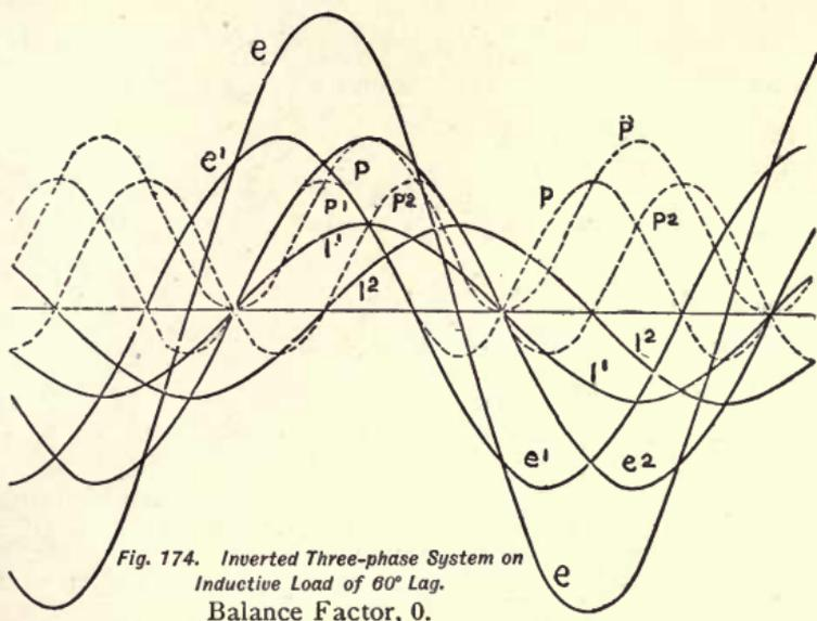
Fig. 174. *Inverted Three-phase System on Inductive Load of 60° Lag. Balance Factor, 0.*
