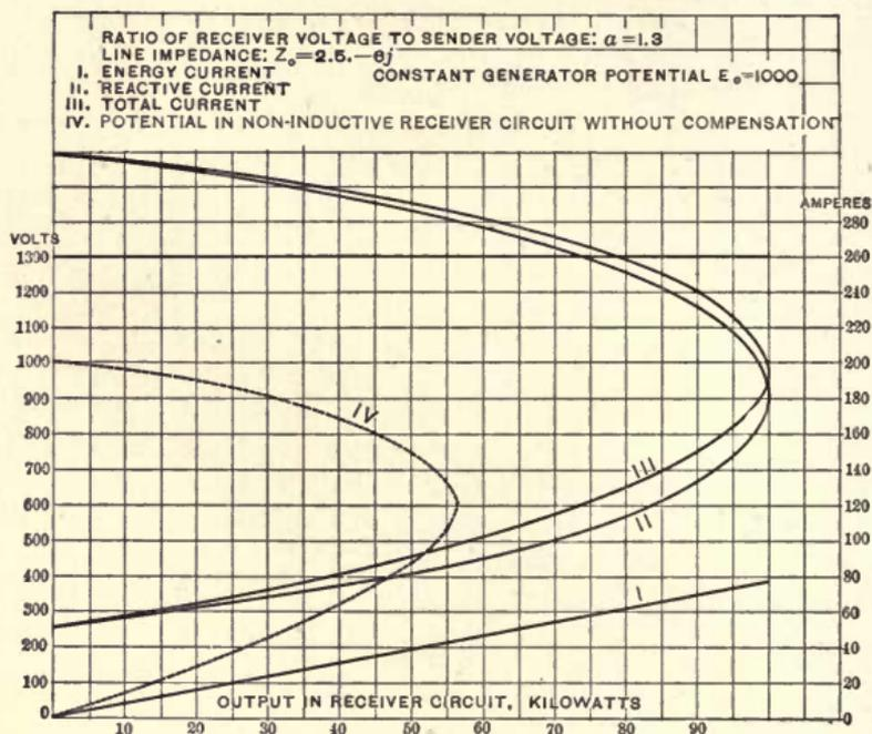
Fig. 63. Variation of Voltage Transmission Lines.
