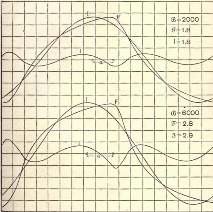
Figs. 66 and 67. Distortion of Current Wave by Hysteresis.
