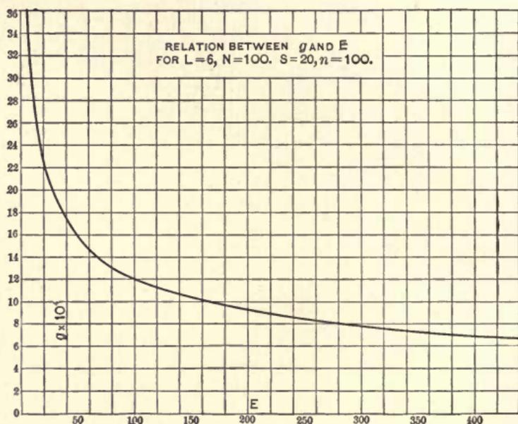
Fig. 76. Hysteresis Conductance as Function of E.M.F.
