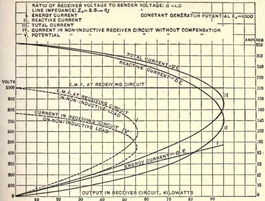
Fig. 61. Variation of Voltage Transmission Lines.
