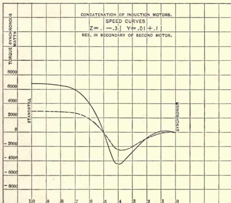
Fig. 125. Concatenation of Induction Motors. Speed Curves.
