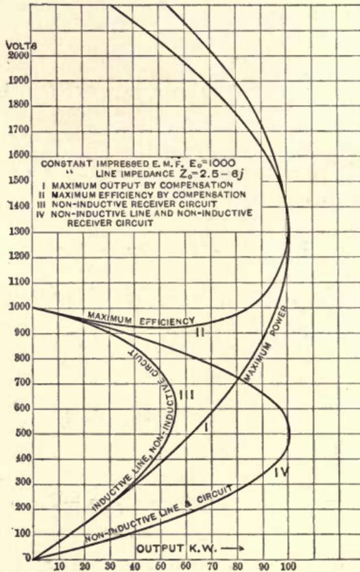
Fig. 64. Efficiency and Output of Transmission Line.
