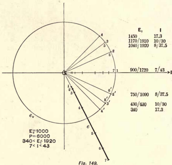
The counter E.M.F. of the motor,  $E_1$ , is  $\overline{OE_1}$ , equal and parallel  $\overline{EE_0}$ , but not shown in the diagrams, to avoid complication.
