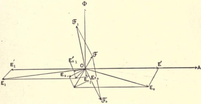
Fig. 101. Transformer Diagram with 80° Lead in Secondary Circuit.
