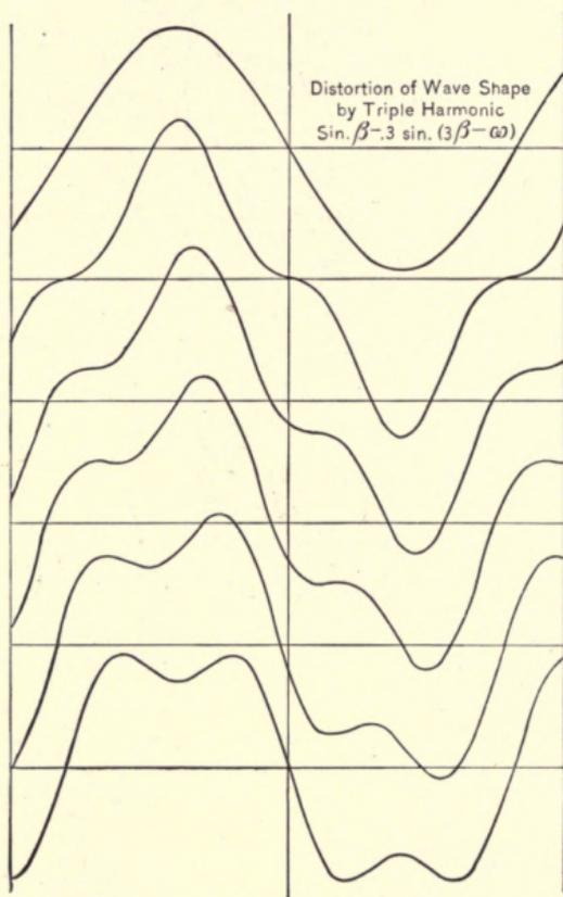
Fig. 175. Effect of Triple Harmonic.
