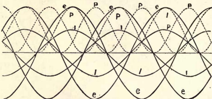
Fig. 189. Three-phase System on Non-inductive Load.
