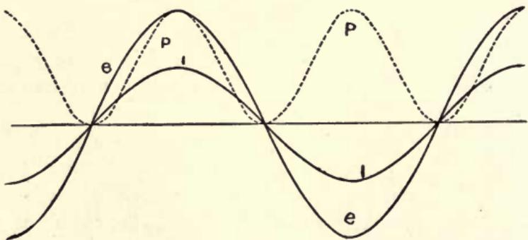
Fig. 185. Single-phase System on Non-inductive Load.
