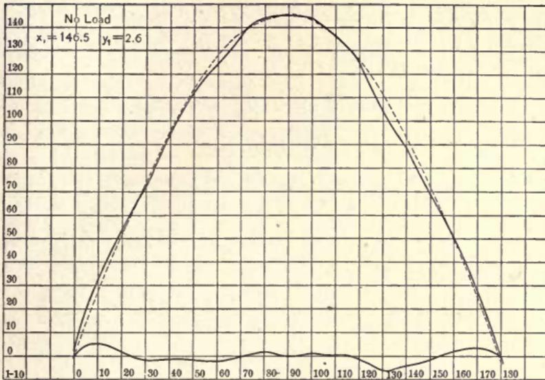
Fig. 169. No-load Wave of E.M.F. of Multitooth Three-phaser.
