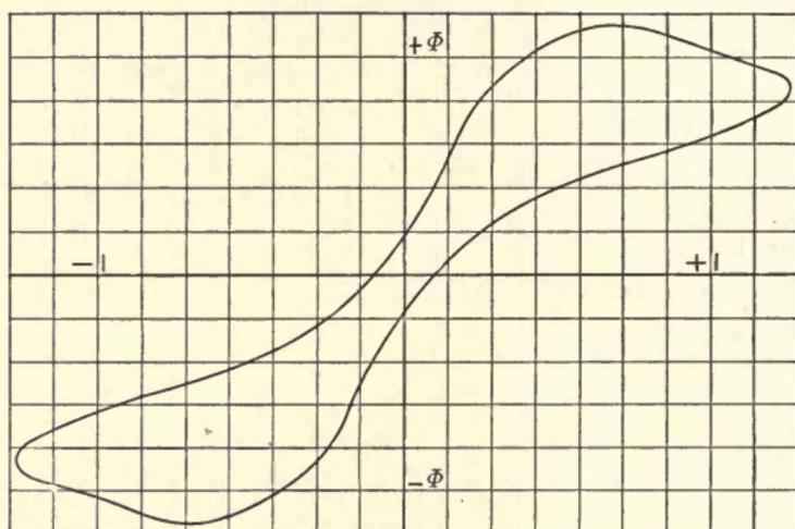
Fig. 167. Hysteretic Loop of Reaction Machine.
