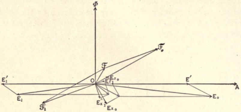
Fig. 97. Transformer Diagram with 20° Lag in Secondary Circuit.
