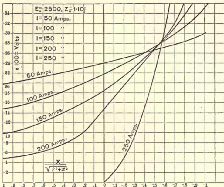
Fig. 135. Regulation of Alternator on Various Loads.
