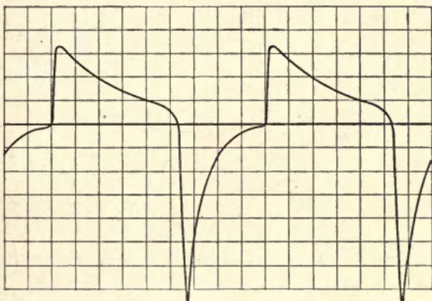
Fig. 3. Wave with Even Harmonics.
