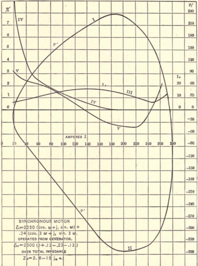
Fig. 180. Synchronous Motor.
