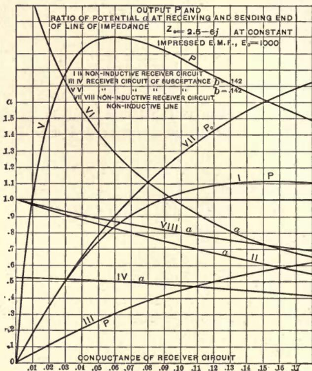
Fig. 58. Variation of the Potential in Line at Different Loads.
