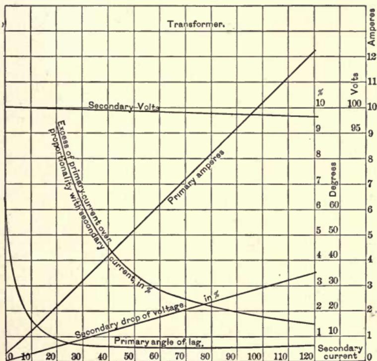
Fig. 110. Load Diagram of Transformer.
