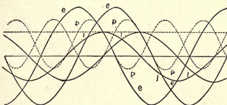
Fig. 188. Quarter-phase System on Inductive Load of  $60^\circ$  Lag.
