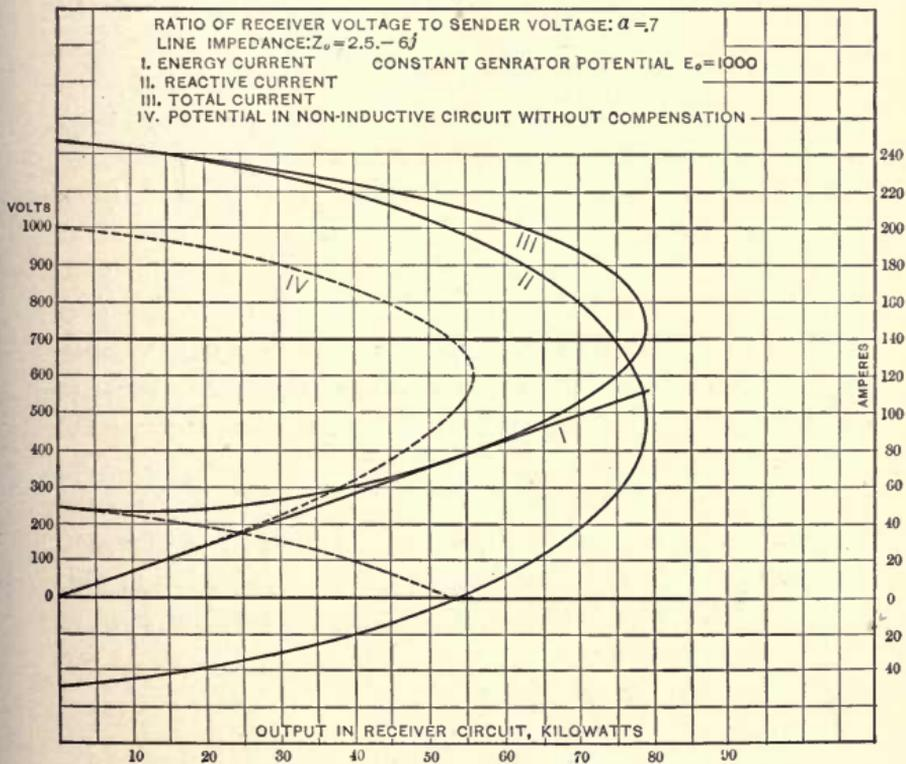
Fig. 62. Variation of Voltage Transmission Lines.
