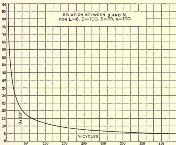
Fig. 77. Hysteresis Conductance as Function of Cycles.
