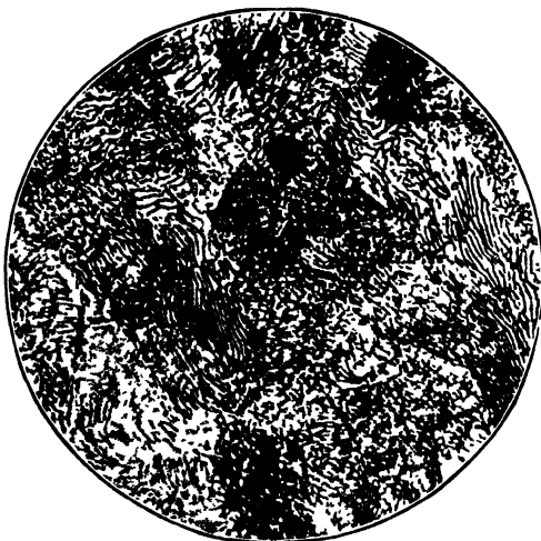
FIG. 7.—Micrograph of pearlite ( \times 500 ).
