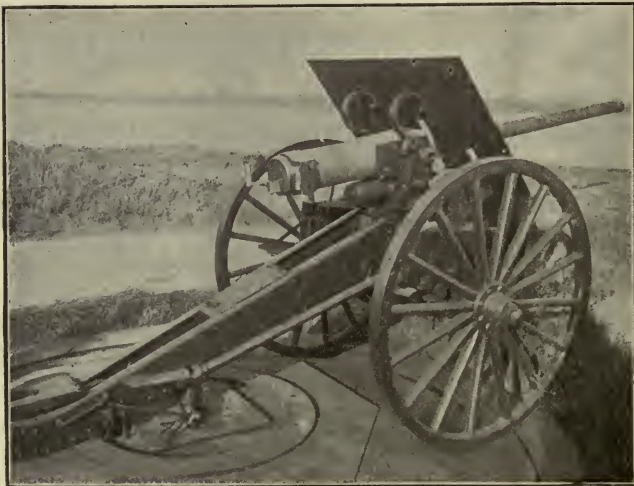
FIG. 16.—2.24-inch (6-pounder) R. F., D.-S. Gun, M. 1900. Interrupted Thread Breech Mechanism. Mounted on Wheeled Mount.
