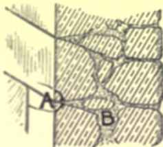
Fig. 32.—Wall-stones with Scamped Beds.
