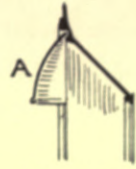
Fig. 65.—Hood inserted in Register-grate.
