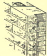
Fig. 35. Window Reveal with Natched Through-stone.
