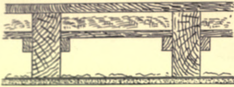
Fig. 88.—Wood Floor and Counterfloor with Lath-and-plaster Ceiling.
