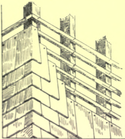
Fig. 54.—Timber-framed Wall covered with Weather-tiling.
