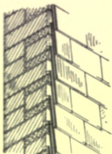
Fig. 57.—Brick Wall with Weather-tiling nailed to Fixing-blocks.
