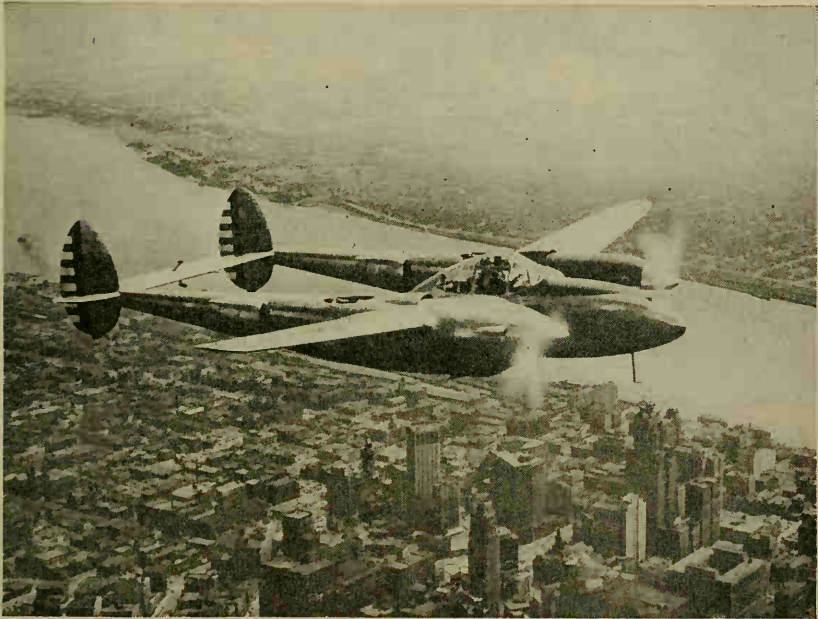
FIG. 148. A P-38 Lockheed interceptor plane which can leave the ground and climb a mile aloft in one minute. Recent tests indicated an airspeed of 458 miles an hour. (Courtesy of the U. S. Army Air Corps.)
