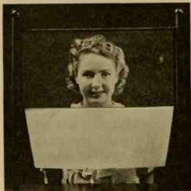
FIG. 290. Two identical sheets of "Louverglas" placed at different angles. Above it appears as transparent sheeting; below it appears translucent. (Courtesy of the E. I. du Pont de Nemours Company.)
