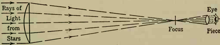
FIG. 3. The principle of the refracting telescope.
