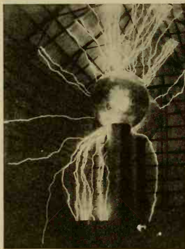
FIG. 234. Artificial lightning produced by the Van de Graaff generator. (Courtesy of the Massachusetts Institute of Technology.)
