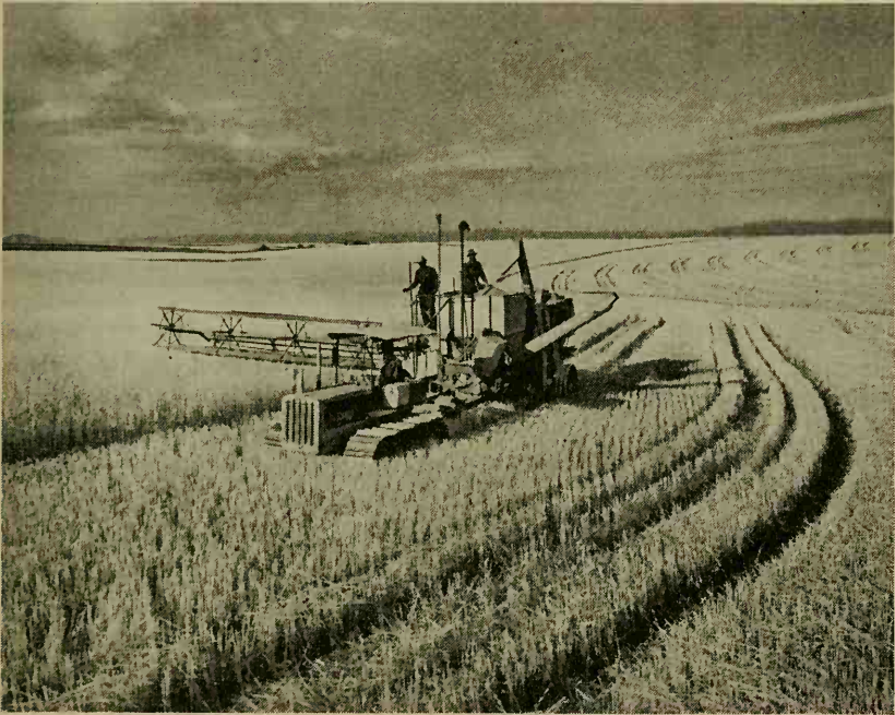
FIG. 141. Caterpillar Diesel pulling a combine, covering 3\frac{1}{2} to 4 acres per hour. Cost of fuel, 9 cents per hour.
