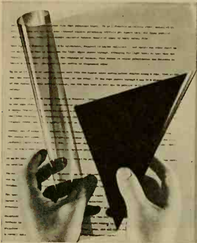
FIG. 188. You can see perfectly through several thicknesses of Polaroid if their "optical slots" are parallel, as they are in the roll at the left. But when the "slots" of the material are crossed, as they are in the fold at the right, no light passes and you cannot see through. (Courtesy of The Polaroid Corporation.)
