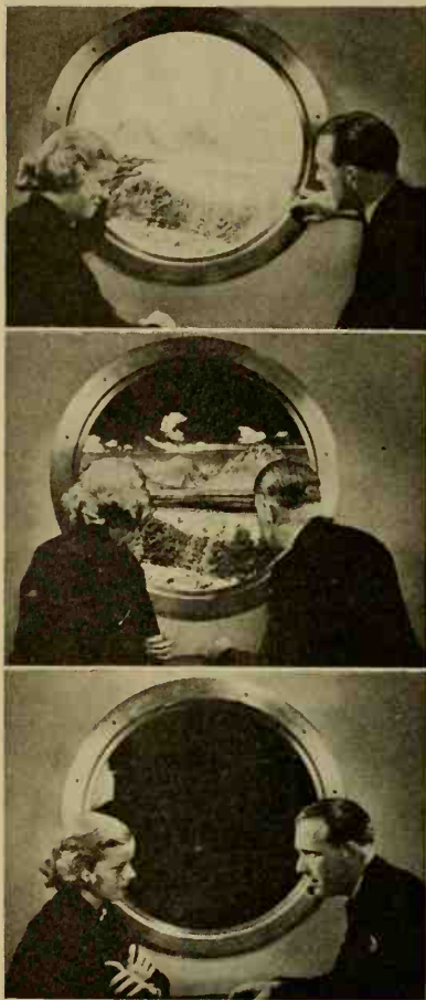
FIG. 199. Control of light in a modern streamliner train by means of a Polaroid screen. (Courtesy of The Polaroid Corporation.)
