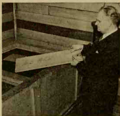
FIG. 287. Removing an oak board from the urea tank. (Courtesy of the U. S. Forest Products Laboratory.)
