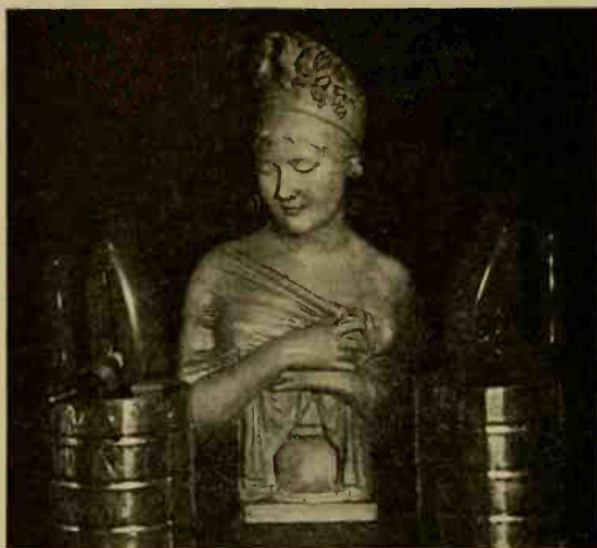
FIG. 170. The irons shown in this figure were heated to produce the infra-red radiations which were used in taking the photograph shown in Figure 171. (Courtesy of the Eastman Kodak Company.)
