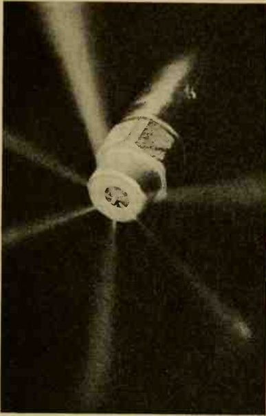
FIG. 140. Photograph of oil spray from an injector.
