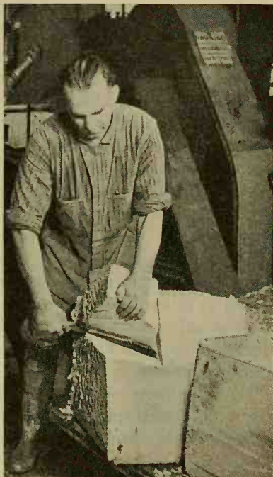
FIG. 307. Cutting a block of raw Ameripol synthetic rubber. (Courtesy of B. F. Goodrich Company.)
