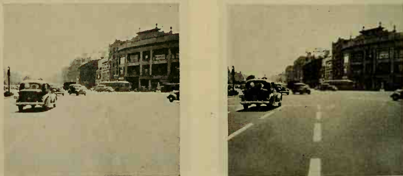
FIG. 192. Left, untouched photograph through ordinary anti-glare glasses. Right, simultaneous photograph identical exposure through Polaroid glasses. (Courtesy of The Polaroid Corporation.)
