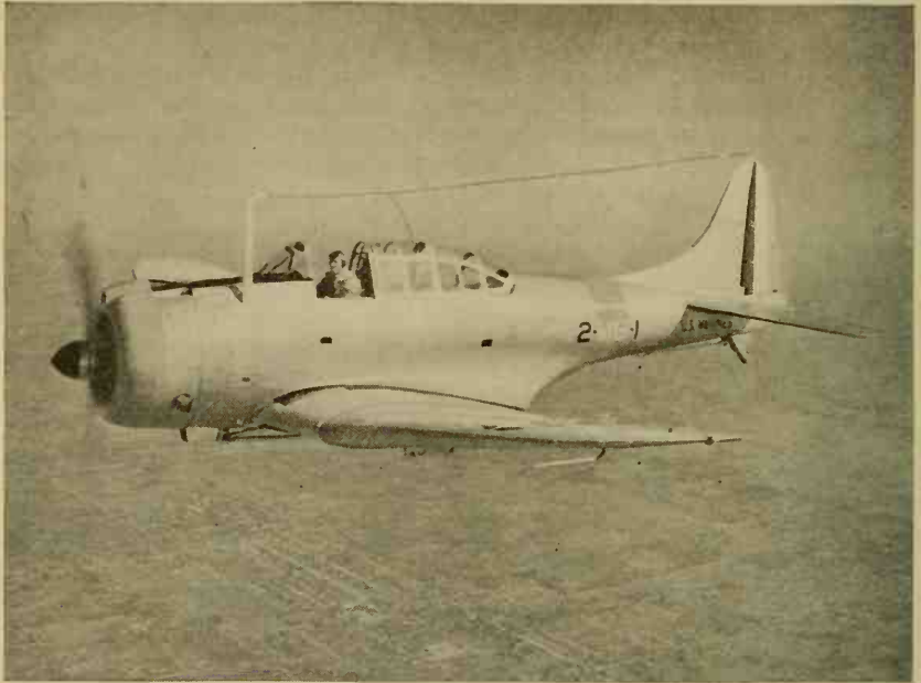
FIG. 149. SBD Douglas dive-bomber. A low-wing type. (Courtesy of the Douglas Aircraft Company.)
