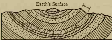
FIG. 50. Tipped strata of rock may be worn away by erosion and left exposed.
