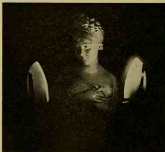
FIG. 171. The photograph obtained using an emulsion sensitized to infra-red radiations. The irons were not hot enough to produce any visible light in the perfectly dark room. (Courtesy of the Eastman Kodak Company.)
