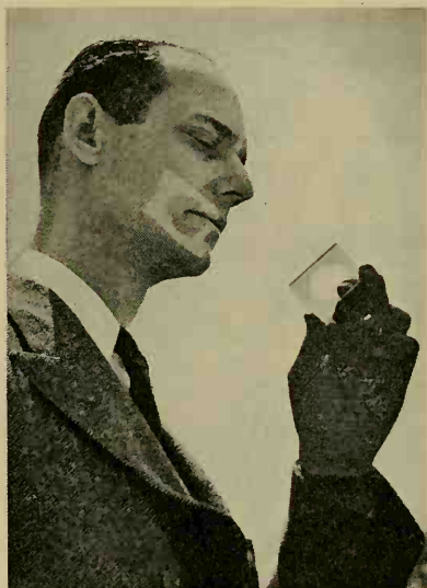
FIG. 203. This reflection on the face of C. Hawley Cartwright shows how a thin film decreases the light reflection from glass. Sunlight is reflected from the glass to his cheek. The round spot in the center of the piece of glass was coated with a thin film of magnesium fluoride. (Courtesy of Science Service.)
