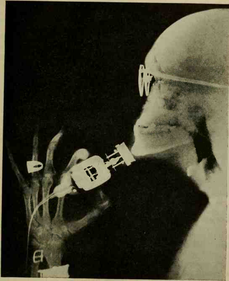
FIG. 272. X-ray radiograph of a man shaving himself, taken with an exposure of 1/1,000,000 second. (Courtesy of the Westinghouse Electric and Manufacturing Company.)
