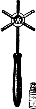
FIG. 5.— Conductometer, an instrument for showing rates of heat transfer in different metals.
